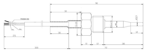
• Wiring Configuration: 2-wire system; shielding wire is not connected to the housing
