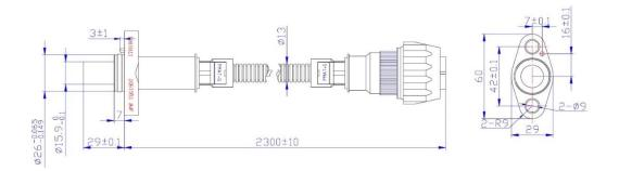
• Electrical Connector: FRCIR06RGG18-20S-F80-V0-M20-1.5F connector, model 27963T12
