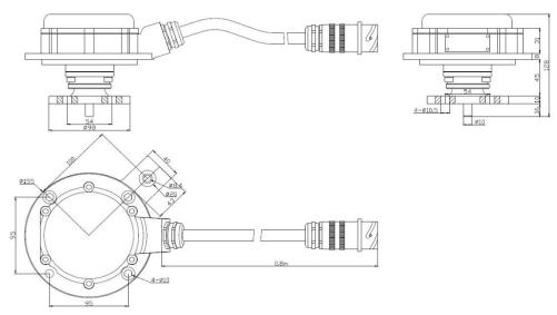
• Electrical Connector: Example configuration — 4 channels, 12-pin connector. Other customized configurations available; please consult technical support.
